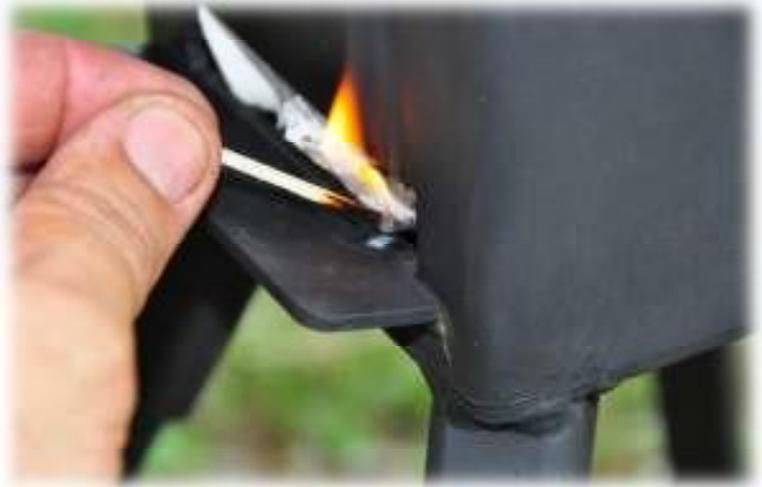
After the fire is started, close the grill and begin inserting small sticks into the front of the stove. Place the sticks only into the fuel feed tube. Do not put sticks into the lower small 1 inch air vent. Allow the fire a minute to start burning all the stick ends and the stove is ready to begin cooking.
